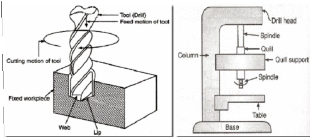
Working Principle of Drill machine Sensitive Drill Machine/Drill Press
