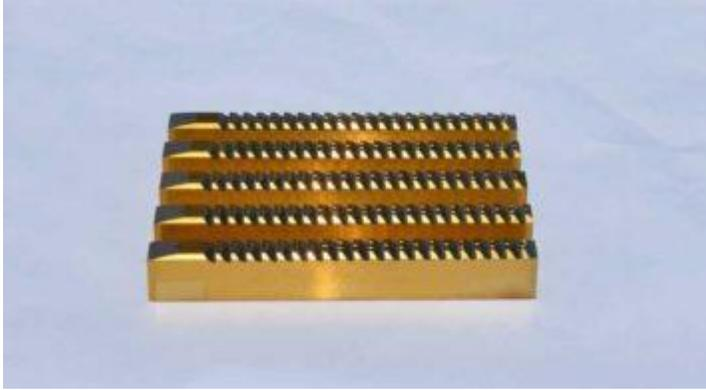
Broaching is a machining process that uses a toothed tool to remove material in a consistent and accurate way. There are two types of broaching services, linear and rotary, which are used to produce different kinds of machining finishes, but in either case, production broaching is typically only used for precision applications and high-quantity production.
